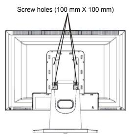
\* Note: Please use UL Listed wall mount bracket with M4 mm x 10 mm (L) screw for application.
